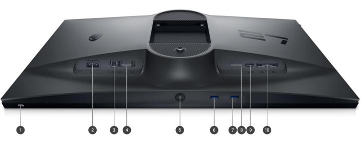
1. Power button | 2. Power connector | 3. USB Type-B upstream port | 4. SuperSpeed USB 5Gbps Type-A downstream port (2) | 5. OSD Joystick | 6. SuperSpeed USB 5Gbps Type-A downstream port with power charging | 7. SuperSpeed USB 5Gbps Type-A downstream port | 8. Security lock slot (based on Kensington Security Slot) | 9. HDMI Port | 10. DisplayPort (2)
