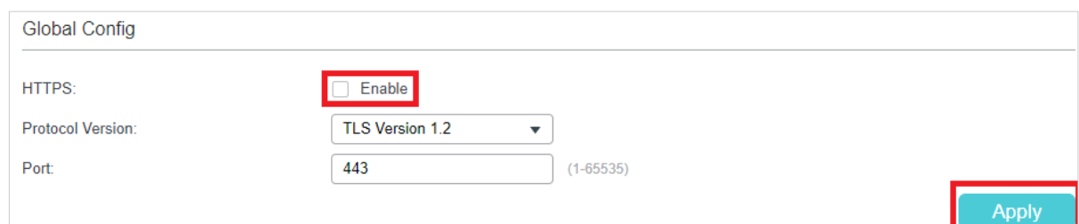
Figure 2-6 Disable the HTTPS Server
