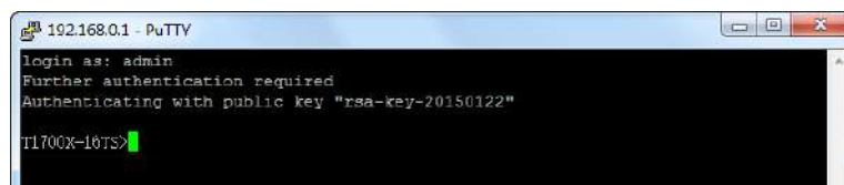
Figure 3-5 Log In to the Switch
