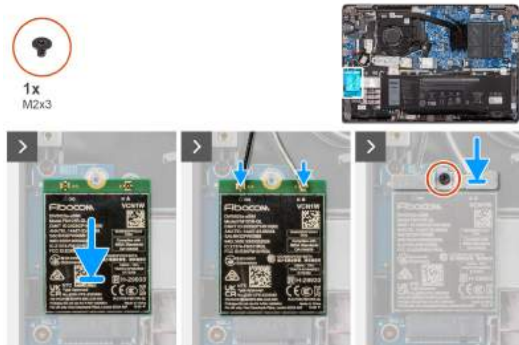
Figure 17. Installing the WWAN card
