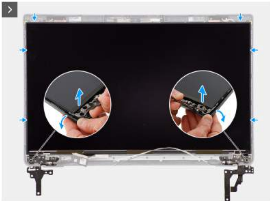
Figure 57. Removing the display panel
