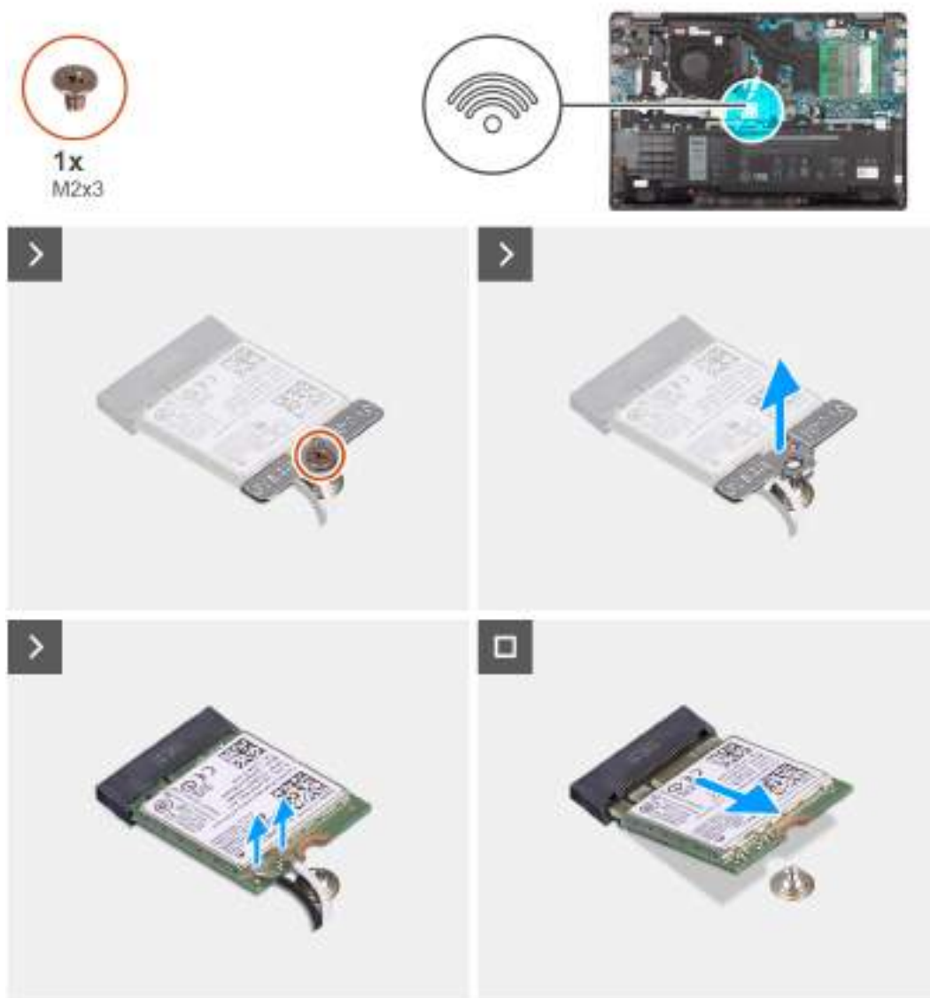
Figure 14. Removing the wireless card
