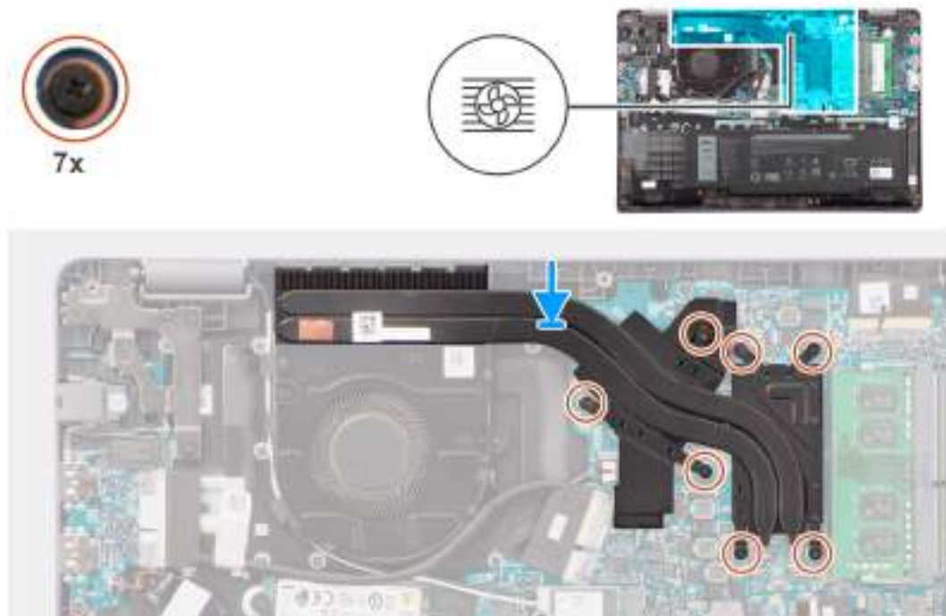
Figure 32. Installing the heat-sink for discrete graphics
