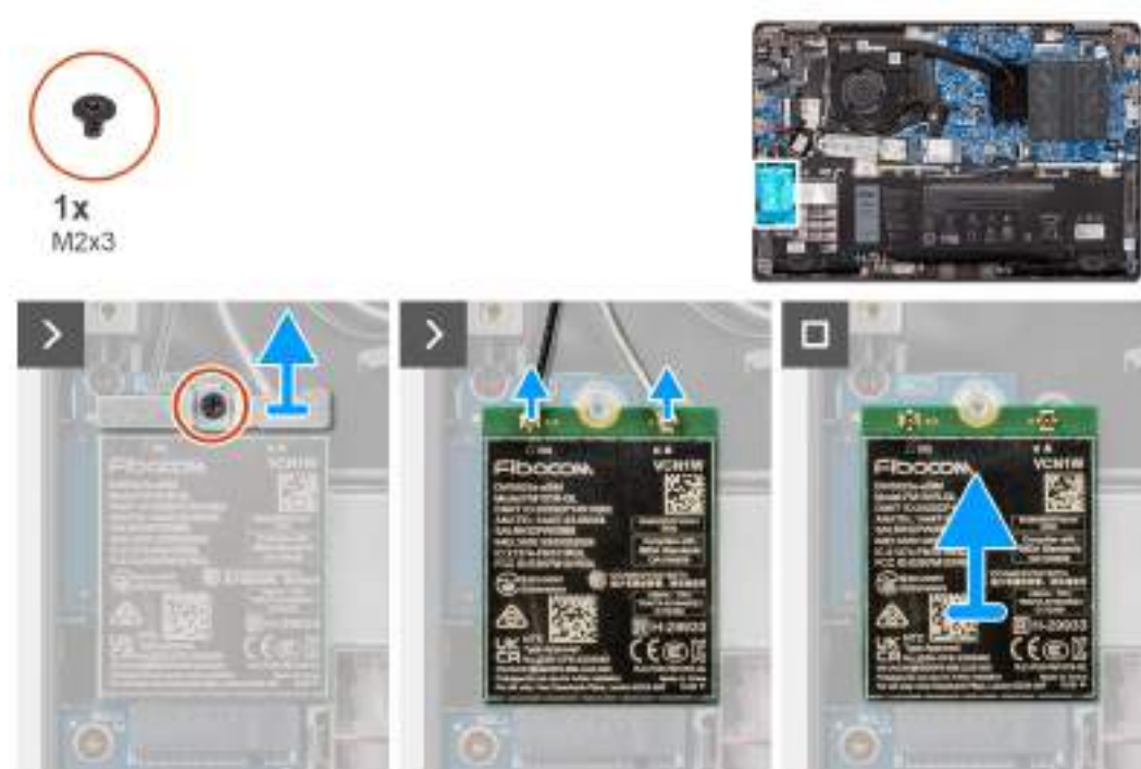
Figure 16. Removing the WWAN card
