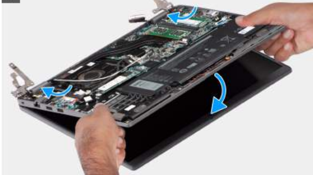
Figure 50. Removing the display assembly
