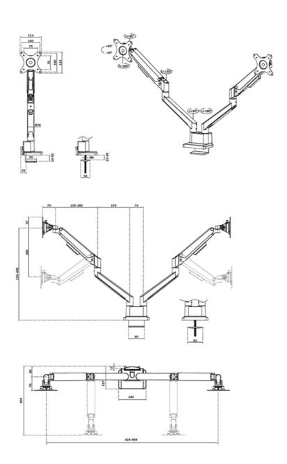
Neomounts Measuring unit: mm
