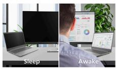
This monitor's PowerSensor 2 feature reduces energy consumption by detecting when users move closer and further away from the screen. After switching the OSD setting to "User", you then need to adjust the settings in Windows 11 for this feature to function properly. When these adjustments are made, the monitor and connected PC/laptop will wake when someone approaches it and sleep when someone walks away, effectively reducing the amount of wake
