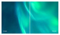
The 10 bit display delivers rich colour depth with 1.07 billion colours and 12 bit internal processing for re-creating smooth, natural colours without gradations or colour banding.
