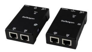
The ST121SHD50 HDMI over Cat5e/Cat6 Video Extender kit lets you extend HDMI video and audio by up to 165 feet (50 Meters) over dual Cat5e cables or dual Cat6 cables. For added versatility the kit features Power Over Cable and only requires a single power adapter that can be connected to either the Transmitter or Receiver.
