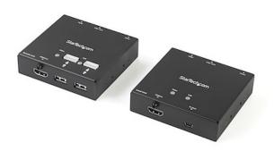
This HDMI extender kit lets you transmit your HD video source to your remote HDMI display at a distance of up to 165 ft. (50 m) away. 1080p video can be extended 131 ft. (40 m) using shielded CAT 6 cabling. The extender features a built-in 4-port USB 2.0 hub that also lets you connect four remote USB peripheral devices at your display location.
